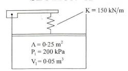
A piston-cylinder device contains 0.05 m<sup>3</sup> of a gas initially at 200 kPa. At this state, a linear spring that has a spring constant of 150 kN/m is touching the piston but exerting no force on it. Now heat is transferred to the gas, causing the piston to rise and to compress the spring until the volume inside the cylinder doubles. If the cross-sectional area of the piston is 0.25 m<sup>2</sup>, determine (i) the final pressure inside the cylinder, (ii) the total work done by the gas.
