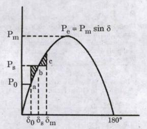
What is the condition of power at point 'b' if  $P_{\rm e}$  is electromagnetic power and  $P_{\rm s}$  is shaft power?
