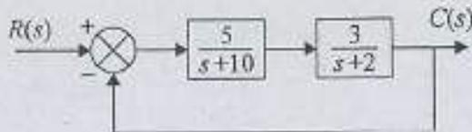
The block diagram shows a unity feedback closed-loop system. The steady-state error in the response to a unit step input is
