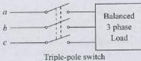
A balanced 3-phase load is supplied from a 3-phase supply. The contact in line  $c$  of the triple-pole switch contactor fails to connect when switched on. If the line-currents in lines  $a$  and  $b$  record 25 A each, then the positive-sequence component of the current is
