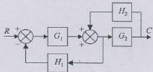
For the block diagram as shown in figure, the overall transfer function  $\frac{C}{R}$  is
