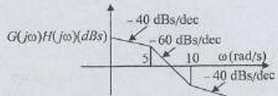
The open loop transfer function  $G(s)H(s)$  of a Bode's plot for feedback system as shown in figure is
