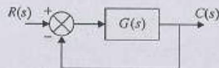
The unity feedback system as shown in the figure is characterized by  $G(s) = \frac{1}{(s+1)^2}$ . The output time response will have a damping factor  $\zeta$ , and natural frequency  $\omega_n$ , respectively, as
