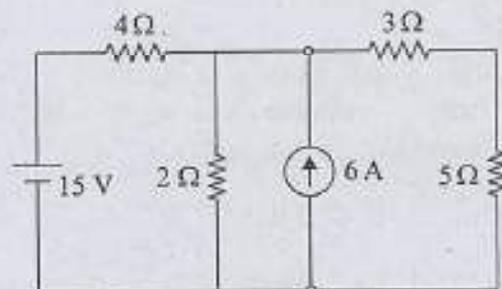
For the network shown in the figure, the current flowing through the  $5\Omega$  resistance will be
