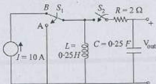
For the circuit as shown, consider that switch  $S_1$  has been in position  $B$  for a very long time and switch  $S_2$  has been open all the time. At time  $t = 0$ , the switch  $S_1$  moves to position  $A$  and switch  $S_2$  closes instantaneously. What is the value of  $V_{out}$  at  $t = 0^+$ , assuming initial charge on  $C = 0$  ?
