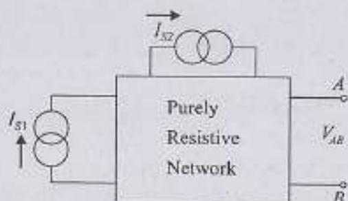
In the network as shown, with  $I_{S1} = 5 \text{ A}$ ,  $I_{S2} = 10 \text{ A}$ ,  $V_{AB} = 120 \text{ V}$ , and with  $I_{S1} = 10 \text{ A}$ ,  $I_{S2} = 5 \text{ A}$ ,  $V_{AB} = 15 \text{ V}$ . What is the value of  $k$  to describe  $I_{S1} = k I_{S2}$ , such that  $V_{AB} = 0$ ?
