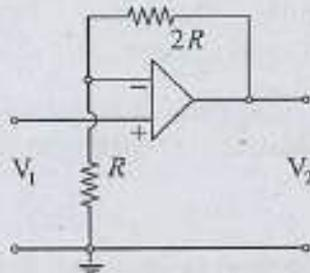
An ideal operational amplifier is connected as shown in figure. What is the output voltage  $V_2$  ?
