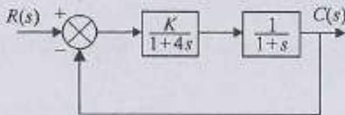
For the feedback control system shown, if the steady state error is 20% for the unit step input signal, then the value of  $K$  must be
