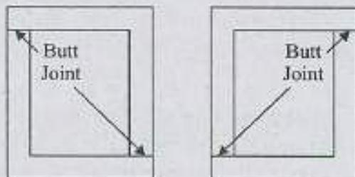
In a core-type single-phase transformer the steel-core is assembled by staggering butt-joints in adjacent layers of laminations vide figures. The purpose served is said to be
