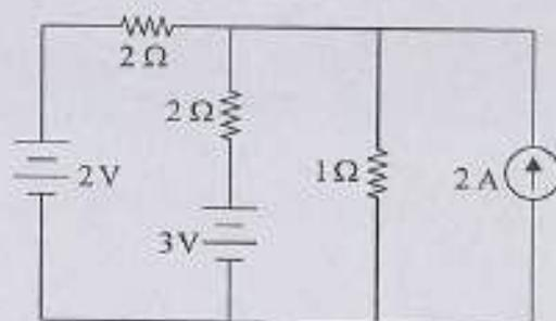
The current in the  $1 \Omega$  resistor in the network as shown is
