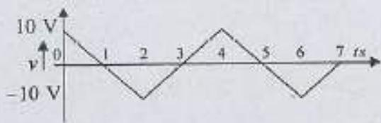
A triangular wave voltage, as shown in figure, is applied across the terminals of a 0.5 F pure capacitor at time  $t = 0$ .
