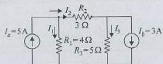
In the circuit as shown, the currents  $I_1$ ,  $I_2$  and  $I_3$  through three resistors are, respectively
