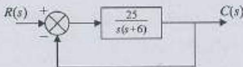
A unit step input to a unity feedback system is shown in the figure, the time for peak overshoot is, nearly
