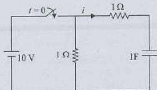
In the circuit as shown in figure, the switch is closed at  $t=0$ . The current through the capacitor will decrease exponentially with a time constant of magnitude
