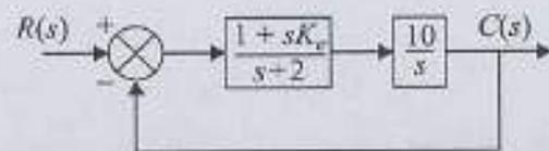
What is the error-rate factor  $K_e$  to yield a damping factor of 0.5 for the system shown in the block diagram?
