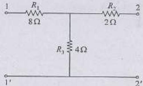
The Z parameters  $Z_{11}$ ,  $Z_{12}$ ,  $Z_{21}$  and  $Z_{22}$  for the circuit as shown in figure, respectively, are
