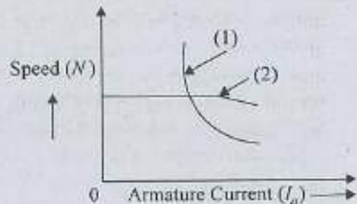
The figure shows plots of speed (N) Vs. armature current ( $I_a$ ) of a dc motor for two different operating conditions. Which one of the following features is relevant?
