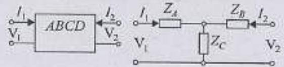
In terms of ABCD-parameters of a 2-port network, the parameters  $Z_A$ ,  $Z_B$  and  $Z_C$  of the equivalent-T-network are, respectively
