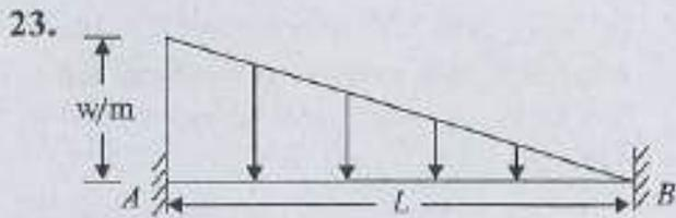
A fixed beam is loaded as in figure. The fixed end moment at support  $A$  is
