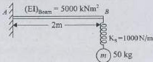
The fundamental time period of vibration of the system shown in the figure, by neglecting the self weight of the beam, is nearly
