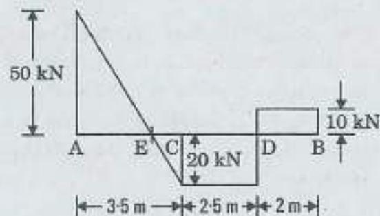
1. The beam ABCD is an overhanging beam having supports at A and D only.
