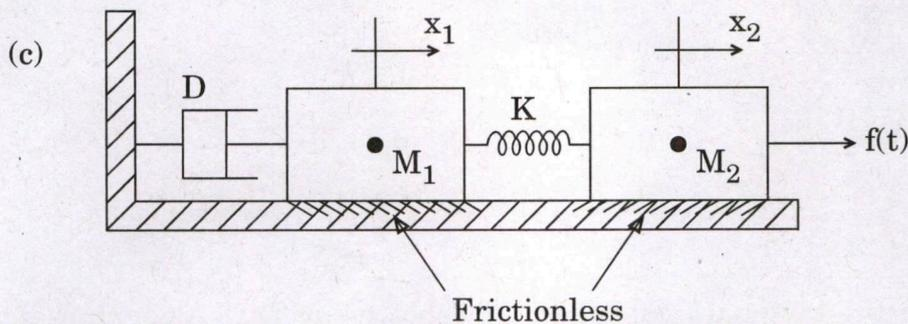
Find the state equations in matrix form for the translational mechanical system as shown above. Assume zero initial conditions, where
