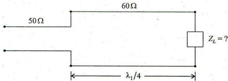
Find the load impedance which can be matched to a  $50\ \Omega$  transmission line with a quarter wave line (at  $f = f_1$ ) of characteristic impedance  $60\ \Omega$ . If the frequency is doubled (at  $f = 2f_1$ ), what will be the VSWR on  $50\ \Omega$  line? 20
