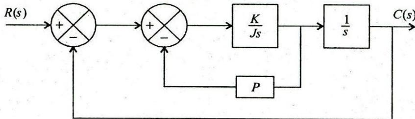
Determine the value of  $K$  &  $P$  of the closed loop system shown in the figure, so that the maximum overshoot in unit step response is 25% and the peak time is 2 sec. Assume that  $J = 1 \text{ kg-m}^2$ . 10
