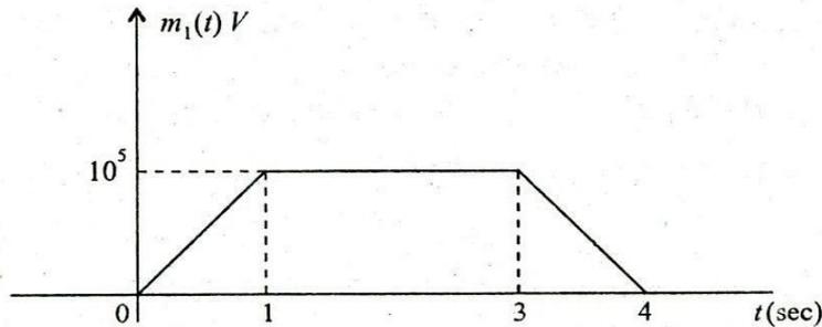
Consider a message signal  $m_1(t)$  as shown and message signal  $m_2(t) = \sin c(2 \times 10^4 t)$ , in volts.
