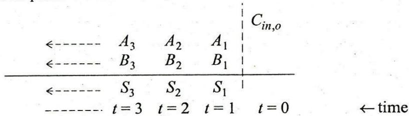
Provision should be made to assert  $C_{in,o}$  as 1 or 0 during the reset pulse. 10
