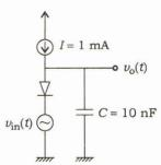
Representing the diode by its small signal resistance  $r_d$ , which is a function of I, sketch the circuit for determining  $v_0(t)$  and thus find out cutoff frequency  $f_H$ . (Assume  $V_T = 25 \text{ mV}$  at room temperature)
