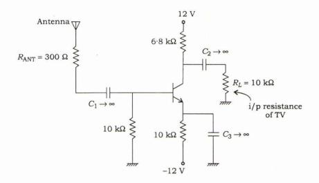
The transistor has high frequency capacitances with  $C_{bc}$  = 4 pF,  $C_{be}$  = 2 pF,  $C_{ce}$  = 1 pF and  $\beta$   $\cong$  100. Calculate low-pass dominant pole frequency and determine whether this amplifier performs adequately. (Assume  $V_T$  = 26 mV at room temperature)
