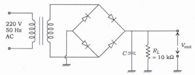
Find the value of C so that the steady current supply to load  $R_L$  can be maintained.
