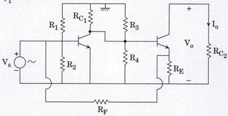
(b) Determine the Z-parameters for the two-port network shown and check for its symmetry and reciprocity.
