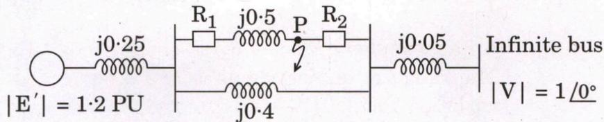
If the generator was delivering 1.0 PU power prior to fault, find the power angle  $\delta$  in pre-fault condition and the maximum permissible angle  $\delta_{\max}$  post-fault after clearing by removing the faulted line by breakers. 12
