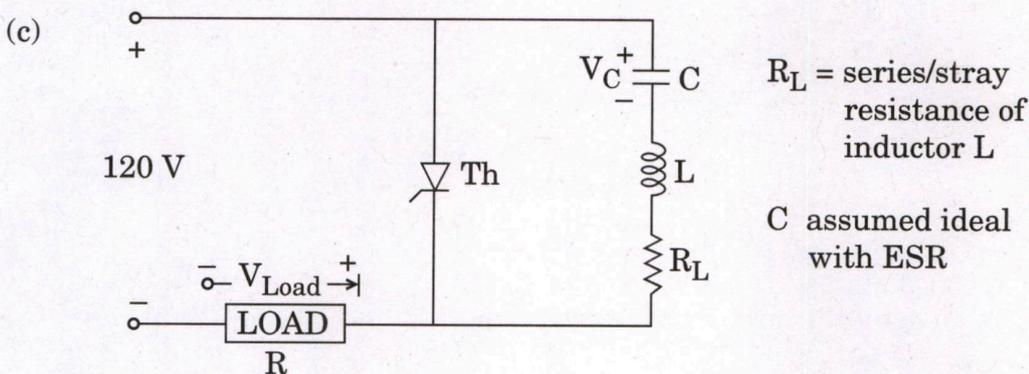
The circuit shown in the figure is in steady state with thyristor OFF for a long time. Find the suitable values of  $L$  and  $C$  for the circuit so that current pulse across the load  $R = 550 \Omega$  is approximately of 1 ms. The circuit is designed to generate a pulse of  $0.75 T$ , where  $T$  is period of resonant circuit. It is assumed that subsequent firing of thyristor occurs after 1 ms and inductor is ideal, i.e.,  $R_L = 0$ . Derive all expressions with  $R_L \neq 0$ .
