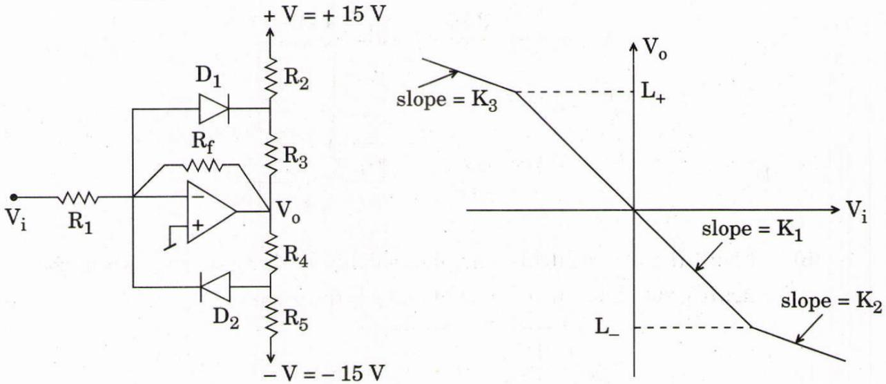
( $R_1 = 30 \text{ k}\Omega$ ,  $R_2 = R_5 = 9 \text{ k}\Omega$ ,  $R_3 = R_4 = 3 \text{ k}\Omega$ ,  $R_f = 60 \text{ k}\Omega$ ).
