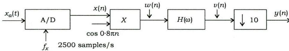
In this system,  $H(\omega)$  is a low-pass filter with a discrete cut-off frequency equivalent to  $f_c = 125 \text{ Hz}$  (normalized w.r.t. the sample rate at the point in the block diagram). Determine and sketch the spectra of  $X(\omega_x)$ ,  $W(\omega_w)$ ,  $V(\omega_v)$  and  $Y(\omega_y)$  w.r.t.  $\omega_x$ ,  $\omega_w$ ,  $\omega_v$  and  $\omega_y$  respectively for  $-\pi < \omega < \pi$ .
