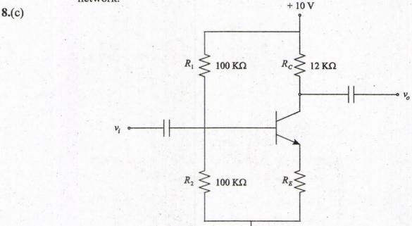
(i) Common emitter (CE) amplifier shown in the figure has voltage gain 400 when  $R_E = 0$ . Stability is brought through negative feedback by adding resistor  $R_E$ . Find the value of resistor  $R_E$  using feedback concepts so that final voltage gain is equal to 200.
