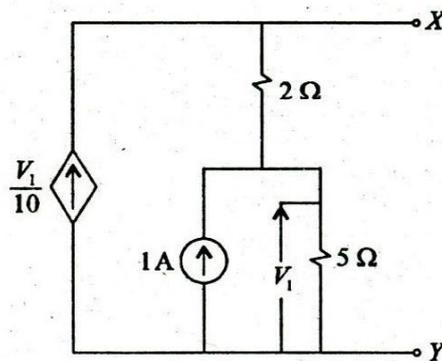
Determine the value of Load Resistance  $R_L$  to be connected across terminals X-Y to receive maximum power. Also, obtain the value of this maximum power.
