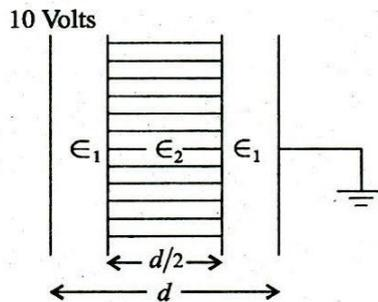
A parallel plate capacitor consisting of two dielectric materials is shown in figure. The middle dielectric slab is placed symmetrically with respect to the plates. If the potential difference between one of the plates and nearest surface of dielectric interface is 4 volts, determine  $\frac{\epsilon_1}{\epsilon_2}$ . Assume parallel plate capacitor has an electrode area of  $A \text{ m}^2$ . 12
