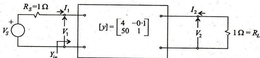
For the two port network shown, the  $y$ -parameter matrix is given.
