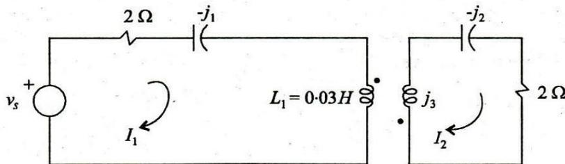
For the network shown,  $v_s = 24\sqrt{2} \sin 100t$ , coefficient of coupling  $k = \frac{1}{3}$  between two coupled coils.
