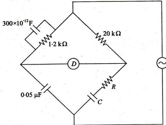
For the bridge circuit shown determine the values of  $R$  and  $C$ . Derive the formula used. 20
