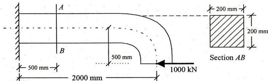
A bracket has been loaded as shown in figure. Compute the top and bottom fibre stress at section A-B.
