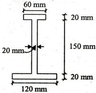
A beam of unsymmetrical I section shown in figure is simply supported over a span of 8 m. It carries a uniformly distributed load of 20 kN/m over the entire span. Draw the sketch for shear stress variation across the depth of the cross-section located at a distance of 3 m from left end A. 20
