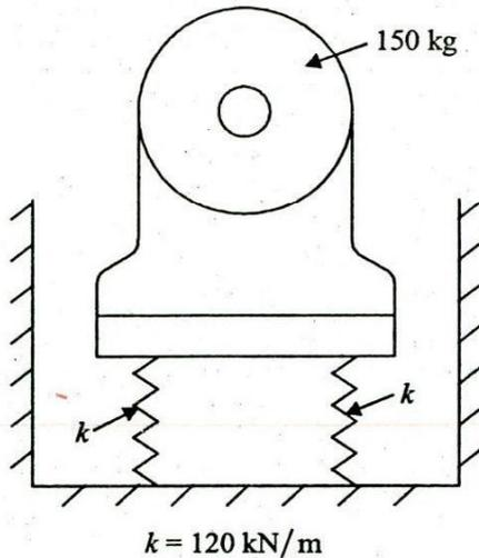
A motor of 150 kg mass is supported by four springs as shown in figure. Each of the springs has a stiffness of 120 kN/m. The unbalance of the rotor is equivalent to a mass of 40 g located at 150 mm from the axis of rotation. The motor is constrained to move vertically. Find
