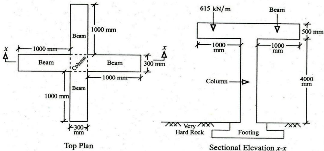
A square column (500 mm × 500 mm) carries load from two beams, which are mutually perpendicular as shown in figure. Overhang portion of beams carry a total load of 615.0 kN/m (include self-weight). Design the column at top of footing level. Footing is fully embedded in very hard rock. Beams are restrained against rotation at Beam-column junction. The minimum eccentricity is less than 0.05 times the lateral dimension of column. Sketch all details required at column cross-section.
