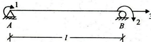
Briefly explain the procedure and then develop the stiffness matrix for the beam element shown in figure with respect to the degrees of freedom 1, 2 and 3. The cross-sectional area  $A$  and flexural rigidity  $EI$  are constant for the beam. 16
