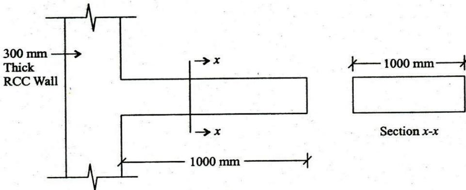
Design a cantilever slab shown in figure for flexure only. Sketch the reinforcement also. Following parameters may be used for design, applying different checks and detailing the reinforcement :
