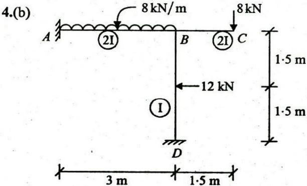
Analyse the frame shown in figure by slope deflection method and draw the B.M.D. and S.F.D. 20
