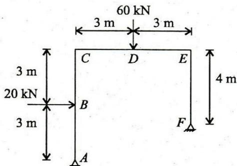
Find the collapse load for a frame of uniform cross-section shown in figure under the applied forces. Also determine the minimum section in steel required to resist the applied forces. 20
