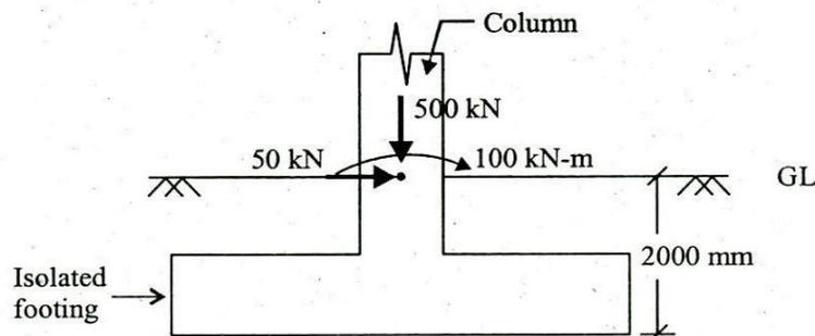
An isolated footing is transferring load from a column (300 mm × 300 mm) as shown in figure. Arrange the plan dimensions of footing so that there will be uniform soil pressure intensity. Following parameters may be used.
