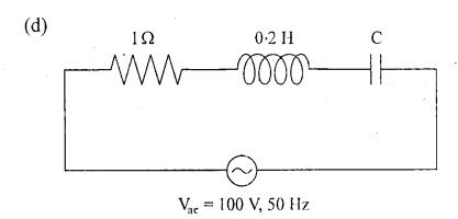
A series RLC circuit with  $R = 1 \Omega$ , L = 0.2 H and an unknown C is excited with an a.c. source of 100 V, 50 Hz. For resonance condition, calculate
