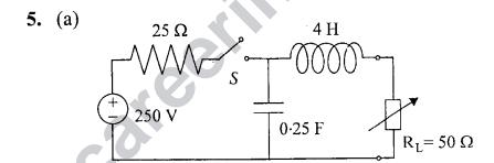
Draw the Thevenin equivalent circuit in the s-domain for the network shown above. Hence find the current through the load,  $R_L = 50~\Omega$  when S is closed.
