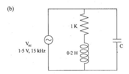
For the circuit shown above, show that the resonant frequency  $f_o = \frac{1}{2\pi} \sqrt{\frac{1}{LC} - \frac{R^2}{L^2}}$ . Calculate C when the supply current is minimum.
