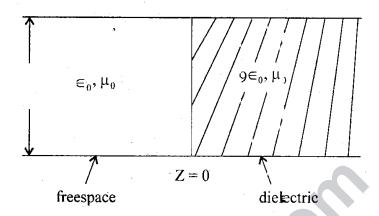
Find the power reflection coefficients for  $TE_{10}$  and  $TM_{10}$  waves of frequency 5 GHz incident on the junction from the free space side. 10
