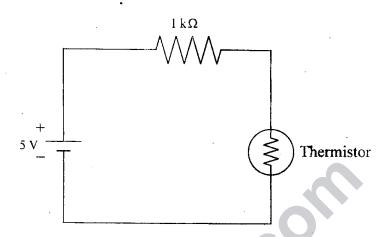
Calculate the Power dissipated in the thermistor shown in the circuit when operated at 150°C. The resistance of the transducer changes as given in the table.
