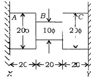
When the temperature of this piece increases by  $50^\circ\text{C}$ , the stresses in sections A and B are
