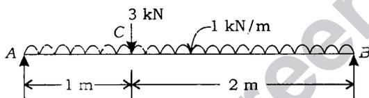
If ISJB 150 with  $I_{XX} = 300 \text{ cm}^4$  is used for the beam, the maximum value of bending stress is
