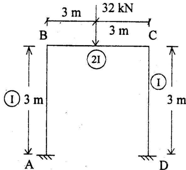
In the rigid frame shown in figure A central concentrated load is acting on "BC". Find slopes
