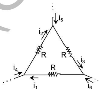
For  $R = 1 \Omega$  and currents  $i_1 = 2 \text{ A}$ ,  $i_4 = -1 \text{ A}$ ,  $i_5 = -4 \text{ A}$ , which one of the following is **TRUE**?
