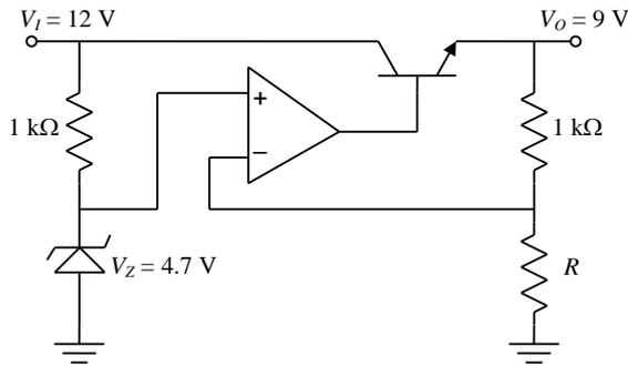
Q.38 In the circuit shown, the op-amp has finite input impedance, infinite voltage gain and zero input offset voltage. The output voltage  $V_{out}$  is
