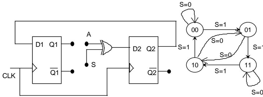
Suppose the XOR gate is replaced by an XNOR gate. Which one of the following options preserves the state diagram?
