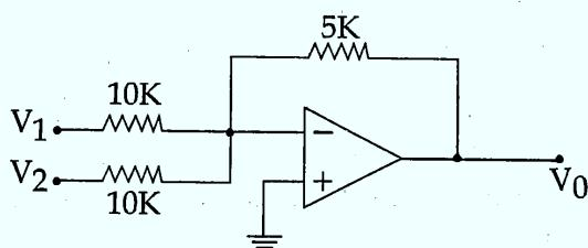
Find the output of the given circuit.
