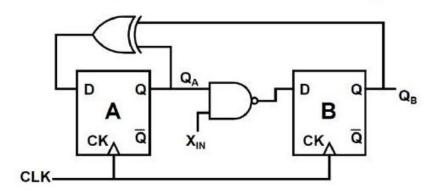
Assume that  $X_{IN}$  is held at a constant logic level throughout the operation of the FSM. When the FSM is initialized to the state  $Q_A Q_B = 00$  and clocked, after a few clock cycles, it starts cycling through
