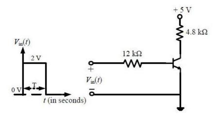
For the input  $V_{in}(t)$  as shown in the figure, the transistor switches between the cut-off and saturation regions of operation, when T is large. Assume collector-to-emitter voltage at saturation  $V_{CE(sat)} = 0.2V$  and base-to-emitter voltage  $V_{BE} = 0.7V$ . The minimum value of the common-base current gain ( $\alpha$ ) of the transistor for the switching should be \_\_\_\_\_\_.
