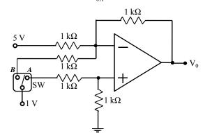
Q.13 In the bistable circuit shown, the ideal opamp has saturation levels of  $\pm 5$  V. The value of  $R_1$  (in  $k\Omega$ ) that gives a hysteresis width of 500 mV is \_\_\_\_\_.
