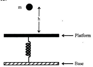
A body of mass m = 1 kg is dropped from a height h = 40 cm on a horizontal platform fixed to one end of an elastic spring, the other being fixed to a base,
