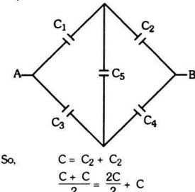
Here, no current will follow the C<sub>5</sub> path because it is null point circuit.
