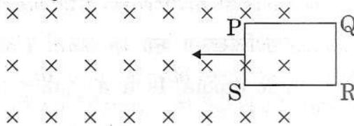
The closed loop (PQRS) of wire is moved into a uniform magnetic field at right angles to the plane of the paper as shown in the figure. Predict the direction of the induced current in the loop.
