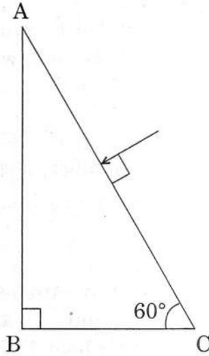
Trace the path of a ray of light passing through a glass prism (ABC) as shown in the figure. If the refractive index of glass is  $\sqrt{3}$ , find out the value of the angle of emergence from the prism.
