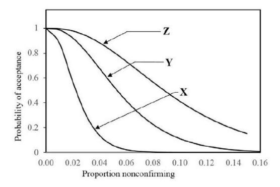
Considering the above operating characteristic curves, the correct relationship of the plans with respect to sample size is
