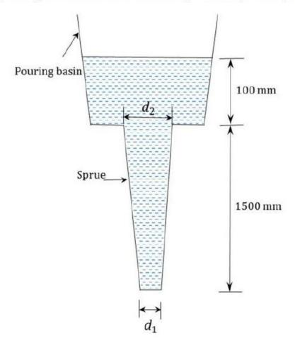
Considering the cross-section of the sprue is circular, the ratio  $d_1$ :  $d_2$  to avoid aspiration is
