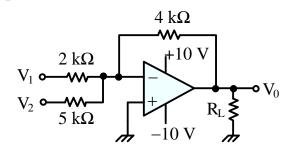
if  $V_1 = 1$  V and  $V_2 = 2$  V, the value of  $V_0$  is \_\_\_\_\_V (up to one decimal place).
