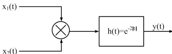
For the system shown above, the minimum sampling rate required to sample  $y(t)$ , so that  $y(t)$  can be uniquely reconstructed from its samples, is
