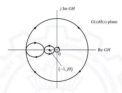
If G(s)H(s) has one zero in the right-half of the s-plane, the number of poles that the closed-loop system will have in the right-half of the s-plane is
