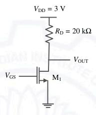
The channel length modulation coefficient is ignored. If the gate-to-source voltage  $V_{GS}$  is 1 V to keep the transistor at the edge of saturation, then the threshold voltage of the transistor (rounded off to one decimal place) is \_\_\_\_\_\_\_ V.
