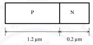
The magnitude of reverse bias voltage that would completely deplete one of the two regions (P or N) prior to the other (rounded off to one decimal place) is  $\_\_\_$  V.
