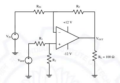
If  $V_{OUT}=1$  volt for  $V_{IN}=0.1$  volt and  $V_{OUT}=6$  volt for  $V_{IN}=1$  volt, where  $V_{OUT}$  is measured across  $R_L$  connected at the output of this OPAMP, the value of  $R_F/R_{IN}$  is
