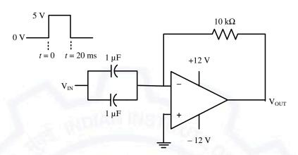
The output voltage  $V_{OUT}$  of this circuit at  $t = 0^+$  (in integer) is \_\_\_\_\_\_V.
