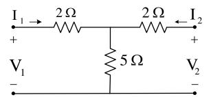
, correct t The parameter B for the given two-port network (in ohms, correct to two decimal places)
