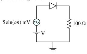
For  $\omega$  = 2×10<sup>6</sup> rad/s, the amplitude of the small-signal component of diode current (in  $\mu A$ , correct to one decimal place) is \_\_\_\_\_.
