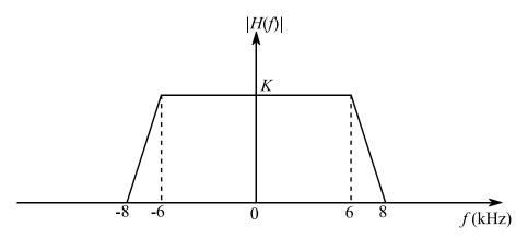
The minimum sampling rate  $f_s$  (in kHz) for perfect reconstruction of x(t) is \_\_\_\_\_.
