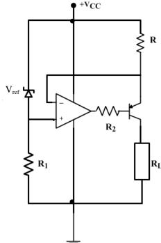
The load current  $I_0$  through  $R_L$  is
